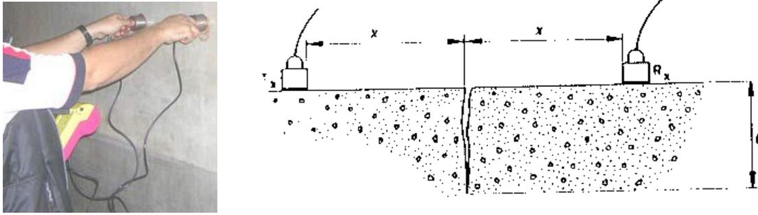
**Figure 21.** Determination of damage to the building by ultrasonic examination, **Source:** Aköz and Yüzer, 2009.
