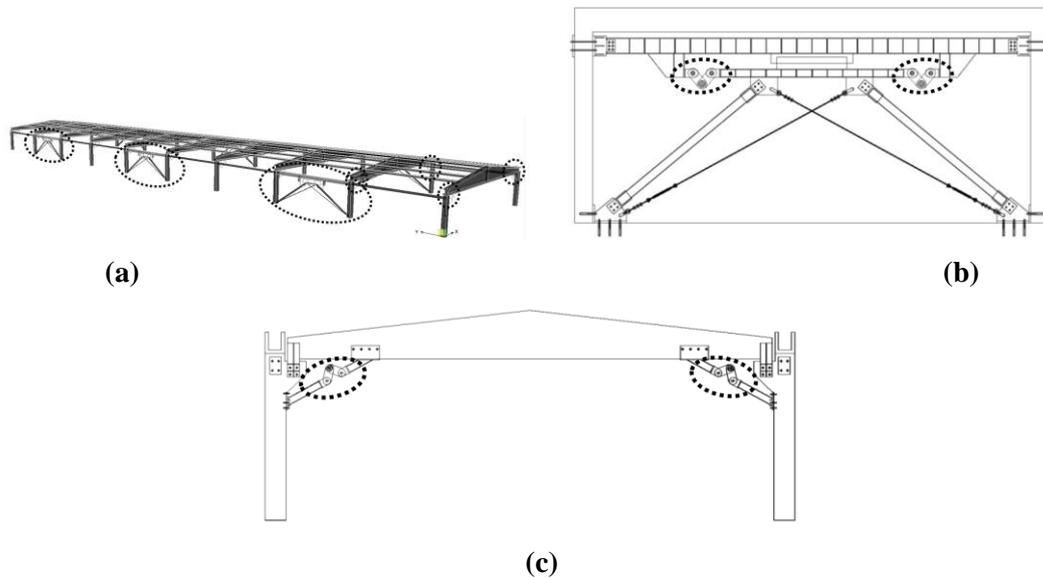
**Figure 13.** (a) Layout of frictional seismic dampers, (b) Inverse V type friction seismic damper placement, (c) Corner junction friction seismic damper placement, **Source:** Yildirim and others, 2015.
