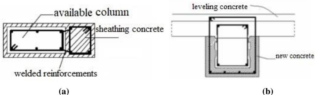
**Figure 1.** (a) Jacket strengthening plan of the column, (b) Strengthening section of the beam, **Source:** Gülmez, 2010.
