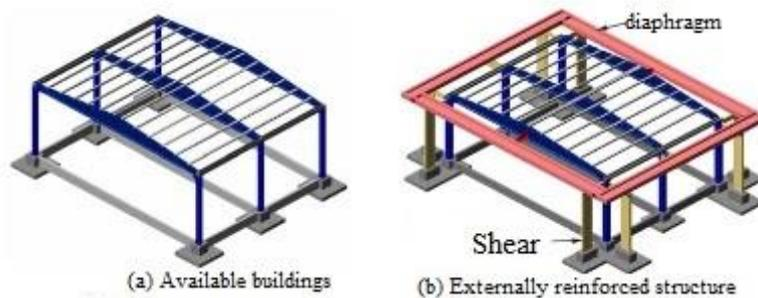
**Figure 14.** Building models reinforced with external shear diaphragm with the existing structure, **Source:** Kaplan and others, 2009.
