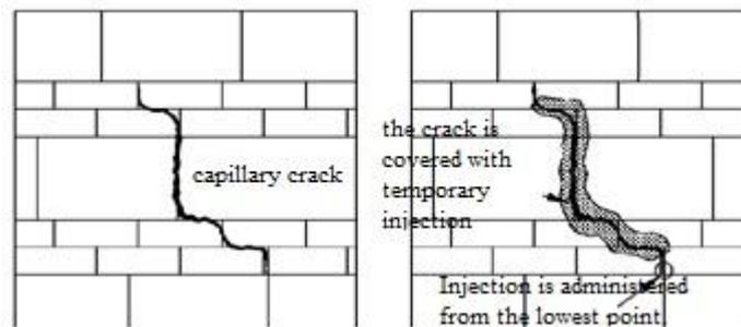
Figure 9. Injection repair of small cracks, Source: Aköz, 2008.
