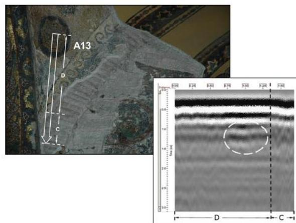
**Figure 20.** GPR scan of the mosaic area unearthed in Hagia Sophia (The target shown by the dashed white curve corresponds to an interior space filled with mortars and bricks), **Source:** Moropoulou and others, 2013.
