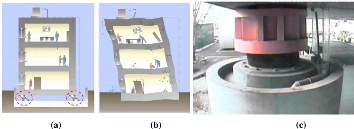
Figure 10. (a) Resistance of the seismic isolated structure against earthquake force, (b) Resistance of the structure without seismic isolation against earthquake force, (c) Seismic isolation application in the building, Source: Nakamura and Okada, 2019.
