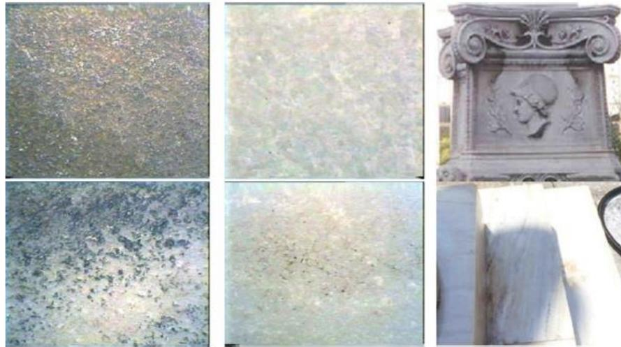
**Figure 22.** Evaluation of the cleaning interventions of the Athens Academy historic building using the fibre optic microscope method, **Source:** Moropoulou and others, 2013.
