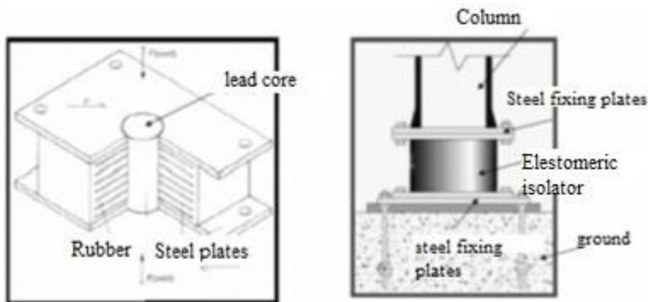
**Figure 12.** Detail of lead core rubber isolator, **Source:** Gülmez 2010.
