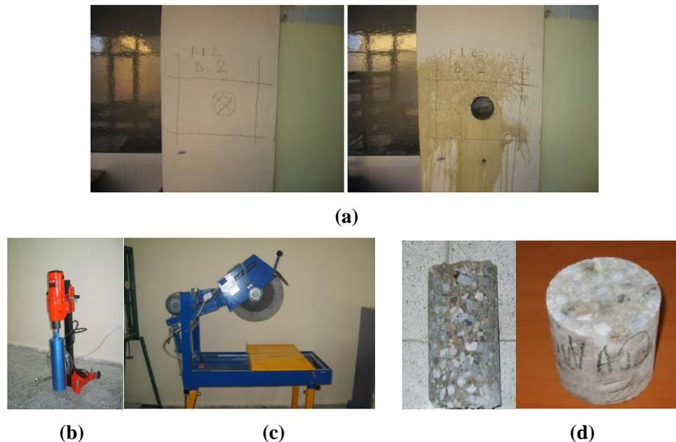
**Figure 16.** (a) Taking the core sample to determine the compressive strength of concrete, **Source:** Kanit and Altın, 2008, (b) Coring tool, **Source:** Altın 2008, (c) The tool used for cutting the core, **Source:** Altın 2008, (d) Extracted and cut core samples, **Source:** Altın 2008.
