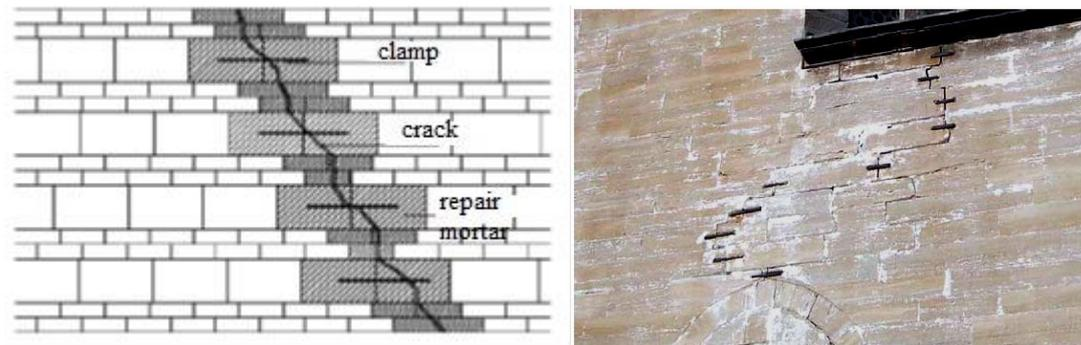
Figure 8. Repairing wide cracks by sewing, Source: Aköz, 2008.
