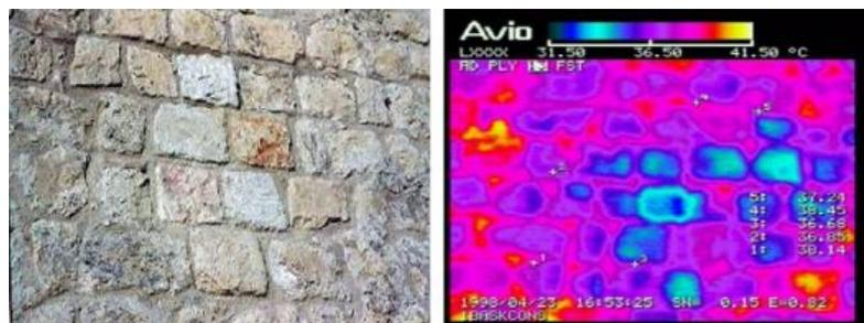
**Figure 19.** Left: Walls facing the National Heraklion Stadium in Crete; Right: Infrared thermography of the same wall, **Source:** Moropoulou and others, 2013.
