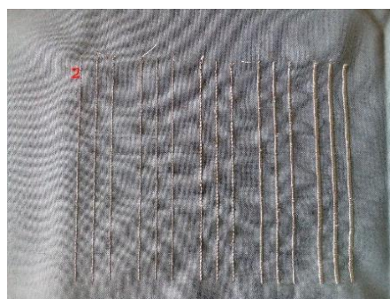
Fig. 14. Stitch Types for Washing Test (Briedis et al, 2019)
